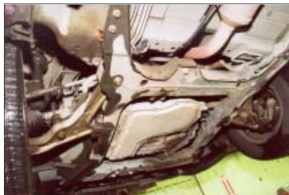
Figure 3: GM consultant's photo of case vehicle's middle and front undercarriage areas viewed from back showing no obvious contacts to undercarriage beyond frontal area (case photo #19)
