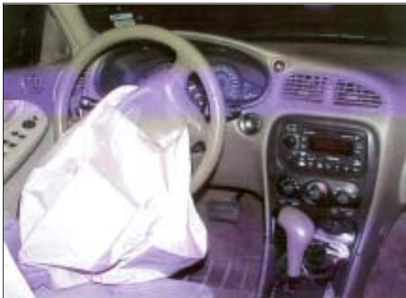
Figure 6: Attorney-provided photo of case vehicle's driver seating area and center console showing deployed driver air bag and no obvious evidence of occupant contact (case photo #02)
