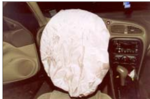
Figure 7: GM consultant's photo of case vehicle's deployed driver air bag showing no obvious evidence of occupant contact (case photo #08)
