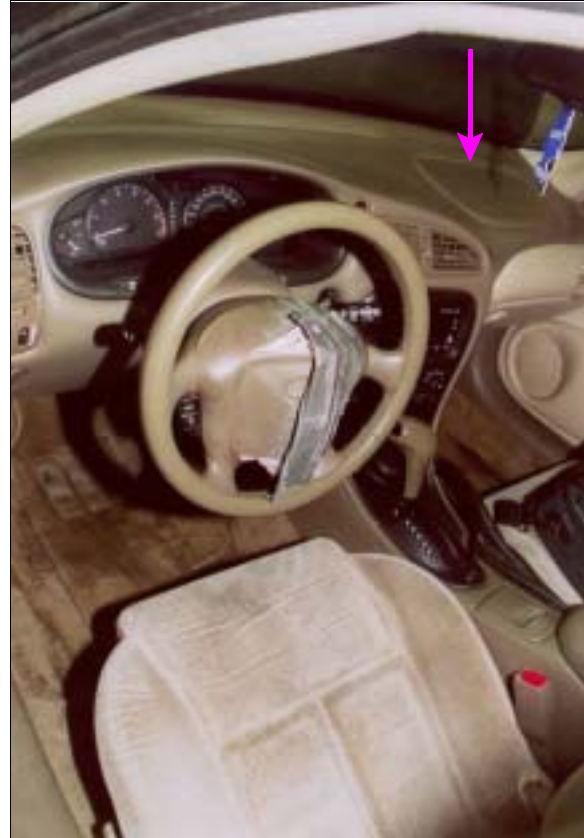
Figure 5: GM consultant's photo of case vehicle's driver seating area showing steering wheel hub from which driver's air bag deployed and non-deployed front right passenger air bag module (case photo #07)
