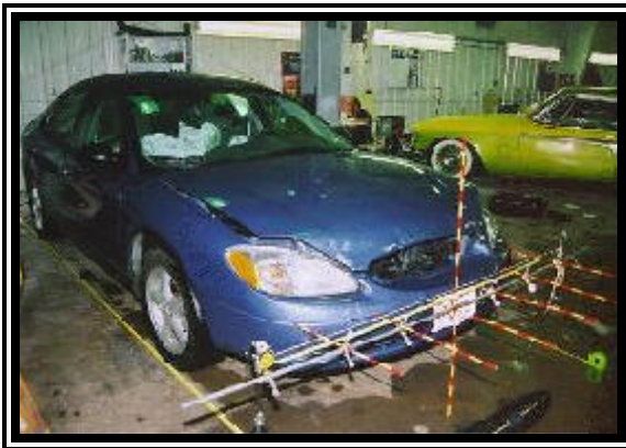
Figure 3. Frontal damage to the 2000 Ford Taurus LX.
