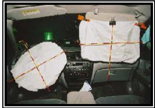
Figure 5. 2000 Ford Taurus LX deployed frontal air bags.
