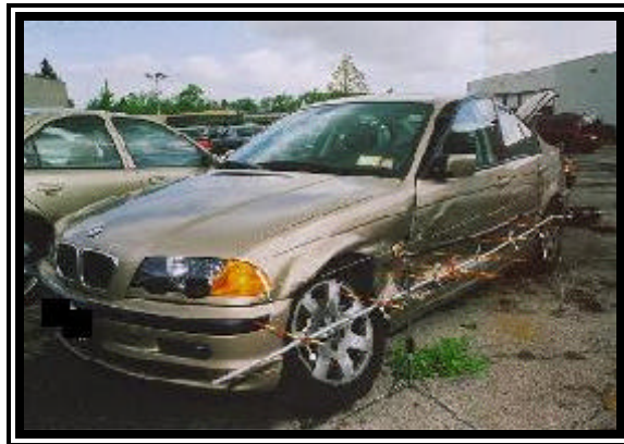
Figure 4. Left side surface damage to the 2001 BMW 325xi.
