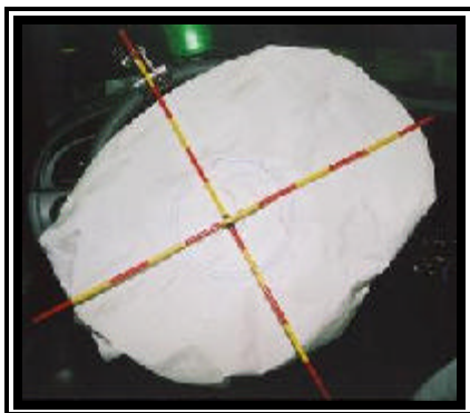
Figure 6. 2000 Ford Taurus LX deployed driver air bag.
