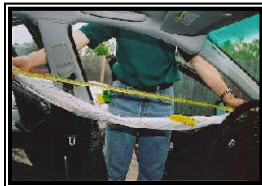
Figure 9. 2001 BMW 325xi deployed head protection air bag.
