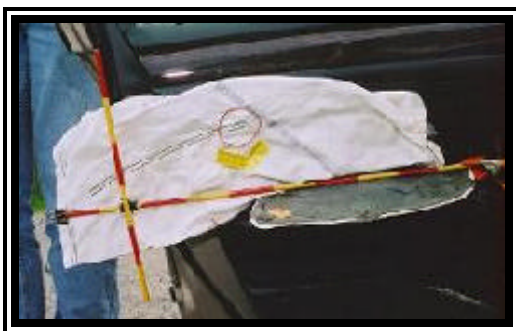
Figure 8. 2001 BMW 325xi deployed left front side impact air bag.
