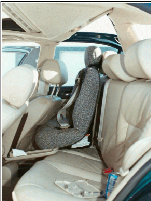
Figure 4: Case vehicle's second seat row, showing intrusion in the area where the booster seat was positioned (case photo #26)
