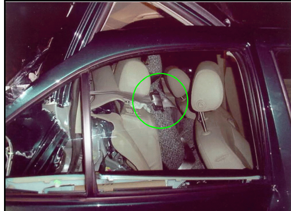
Figure 8: On-scene view of right rear seat position, looking through right rear door window; note vehicle's shoulder belt threaded through booster seat's positioning guide clip (highlighted) (case photo #63)
