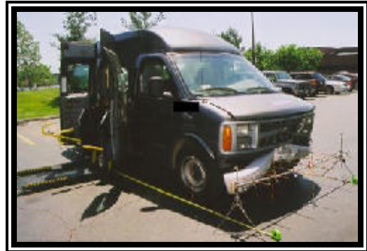
Figure 3. Frontal damage to the 2000 Chevrolet G2500 Express van.
