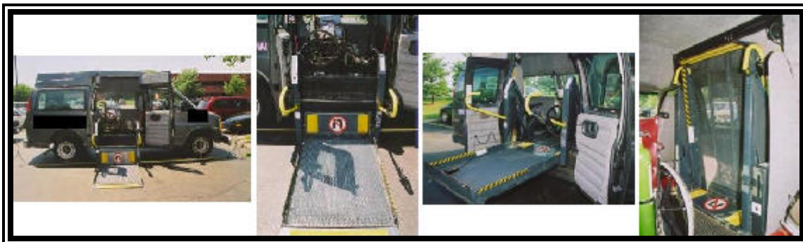
Figure 5. Wheelchair lift system in the down and retracted position.
