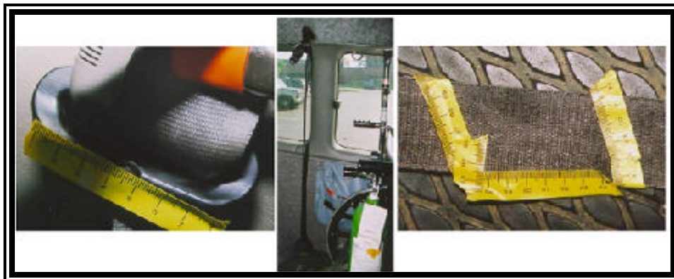
Figure 7. Loading evidence to the driver's D-ring and rear left manual lap belt.
