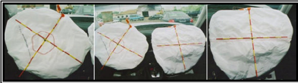
Figure 7. 2001 Volkswagen Jetta deployed redesigned frontal air bags.
