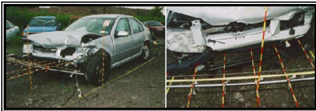
Figure 4. Front left damage to the 2001 Volkswagen Jetta.
