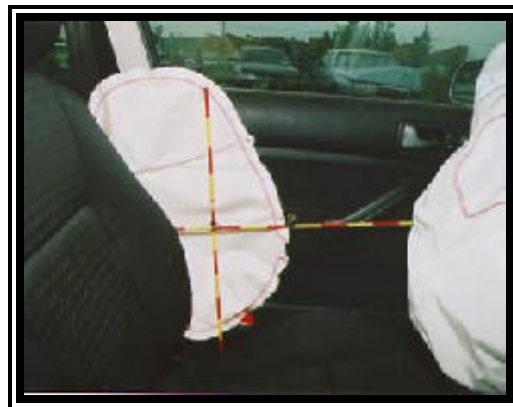
Figure 8. 2001 Volkswagen Jetta deployed driver side impact air bag.
