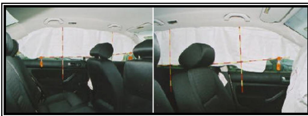
Figure 9. 2001 Volkswagen Jetta deployed left side impact curtain.
