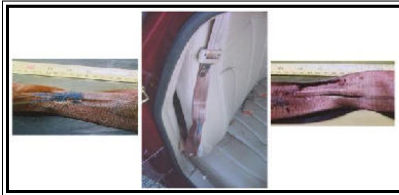
Figure 10. Loading evidence and fabric transfers to the rear right 3-point manual restraint.
