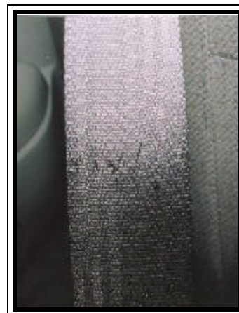
Figure 17. Loading evidence on the rear right shoulder harness.
