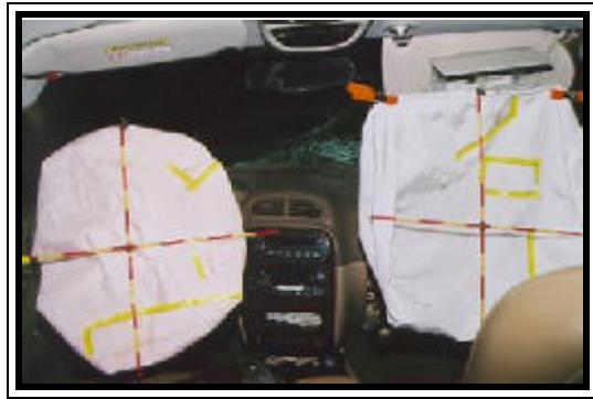
Figure 12. 2000 Chrysler Concorde deployed redesigned frontal air bags.
