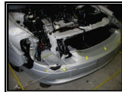
Figure 7. Damaged radiator supports
