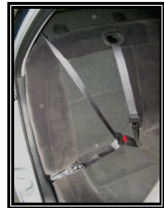
Figure 9. View of creases in the rear right belt webbing
