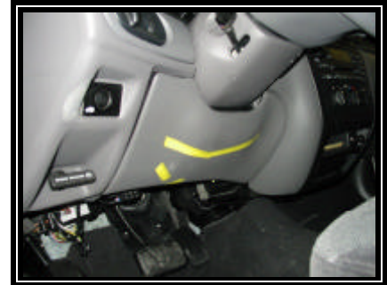
Figure 8. View of displaced and scuffed knee bolster
