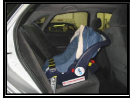
Figure 12. Right side view of installed CSS showing sticker with horizontal arrow
