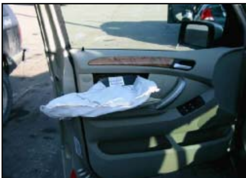
Figure 10. Deployed door panel mounted side impact air bag.
