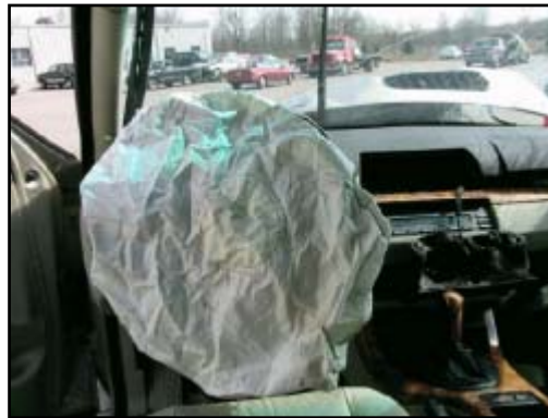
Figure 9. Deployed front left air bag.
