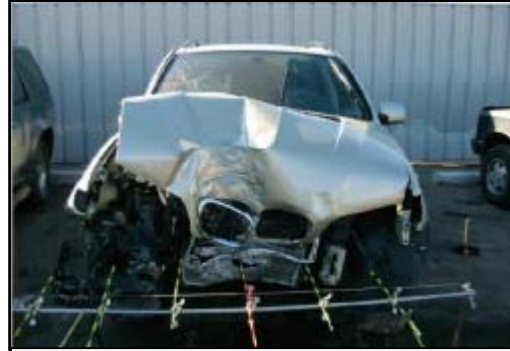
Figure 1. Front damage to the BMW X5 sport utility vehicle.
