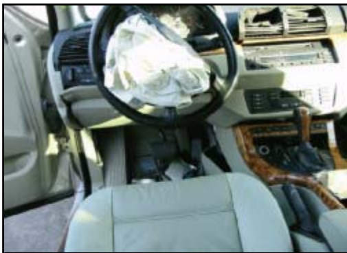
Figure 6. Deformed steering wheel rim and occupant contact lower left knee bolster.
