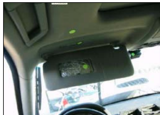
Figure 5. Occupant contact to sunvisor and headliner.
