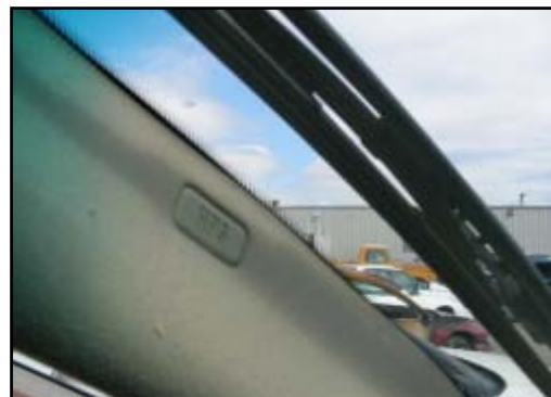
Figure 11. Identification acronym for the non-deployed HPS at the left pillar.
