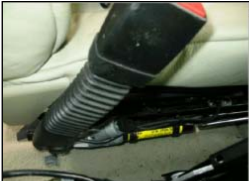
Figure 8. Non-fired status of the front left buckle pretensioner.
