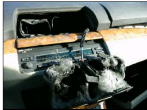
Figure 7. Fire damage to center instrument panel.
