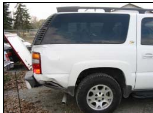
Figure 7. Close-up of right rear sideslap damage
