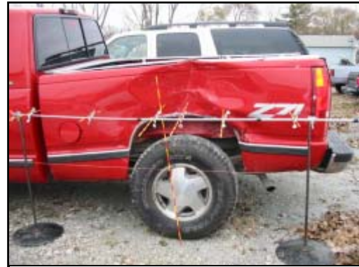
Figure 10. Left rear damage from the sideslap event
