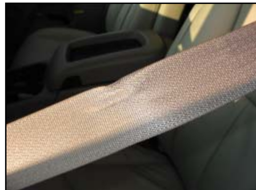
Figure 11. View of deformed driver's safety belt webbing
