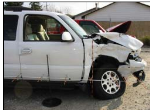
Figure 6. View of right front crush measurements
