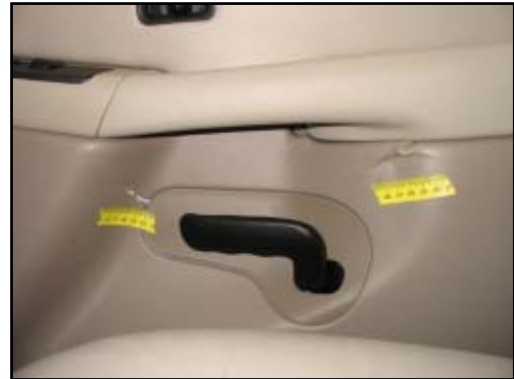
Figure 8. View of occupant contact to the interior right front door
