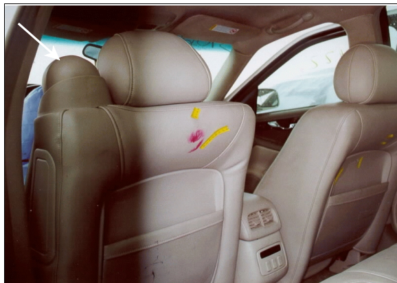
Figure 7: Lipstick imprint on back surface of case vehicle's driver seat back from contact by back left passenger; Note: driver's seat integrated restraint system (case photo #49)
