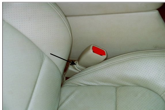
Figure 15: Close-up of buckle for case vehicle’s front right passenger seat belt system showing actuated pretensioner (case photo #42)
