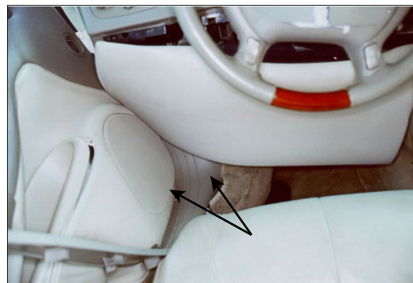
Figure 9: Overhead view of case vehicle's driver seating area showing lateral intrusion into area (case photo #33)
