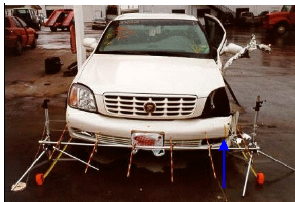
Figure 4: Elevated view of case vehicle's frontal damage with contour gauge present at bumper level; Note: yellow tape (arrow) marks width of direct damage on bumper (case photo #06)
