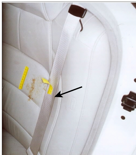
Figure 16: Close-up of case vehicle's back left seat belt system showing loading evidence on belt webbing (i.e., yellow tape) and blood evidence on seat back's cushion (case photo #47)
