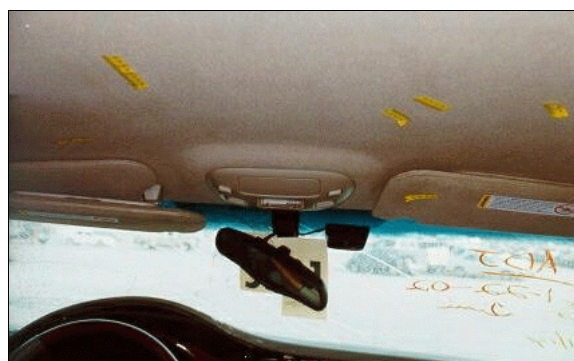
Figure 6: Case vehicle's roof and windshield header areas showing hair deposits on roof over both front passenger positions, hair deposit on front right sun visor, and a scrape over driver's position (case photo #28)
