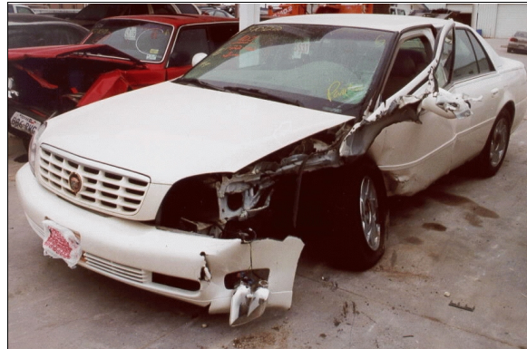
Figure 2: Case vehicle's front left damage viewed from left of front; Note: direct damage continues down left side and involves left outside rearview mirror and left front wheel was displaced rearward (case photo #08)
