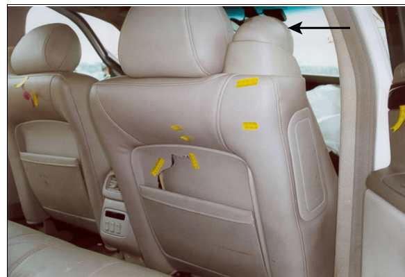
Figure 8: Fracture and contact evidence on back surface of case vehicle's front right passenger seat back from contact by back right passenger; Note: front right passenger's seat integrated restraint system (case photo #51)
