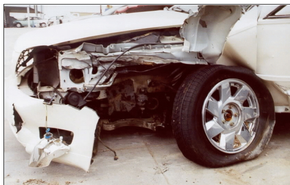
Figure 5: Case vehicle's front left damage viewed from left; Note: left front tire and wheel assembly were crushed rearward and separated from front axle, tire rod, steering arm, and suspension (case photo #11)
