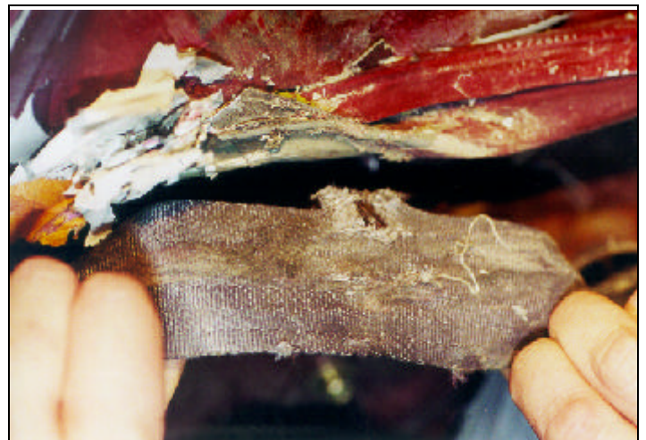
Figure 20. Tearing damage from torn metal.
