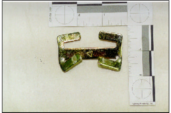
Figure 18. Deformed locking clip for right side child seat.
