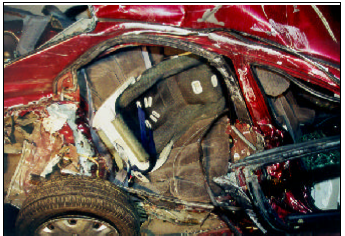
Figure 14. Final position of left rear child seat.
