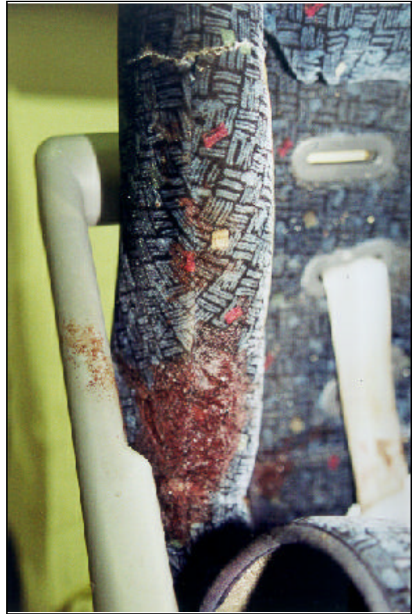
Figure 12. Right side of Century child seat showing shell fracture.
