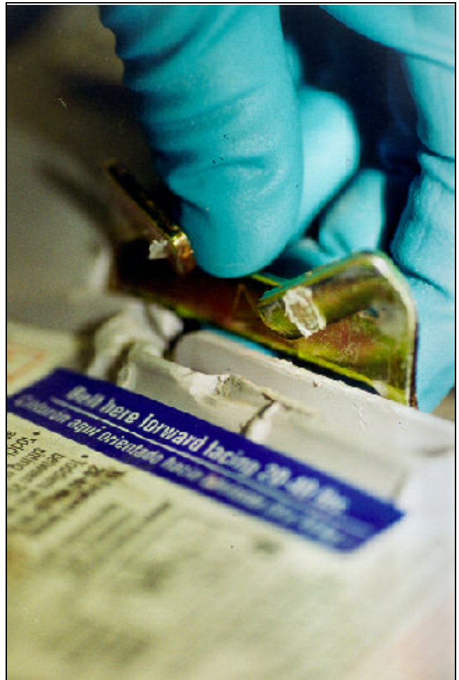
Figure 21. Locking clip damage.
