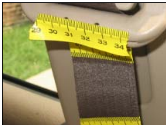
Figure 12: Close-up view of scuffing/friction burn on seat belt of case vehicle's driver (case photo #36)
