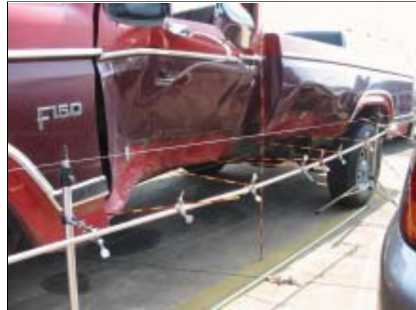
Figure 4: Ford pickup's left side damage—with contour gauge at sill level, resulting from impact with case vehicle; Note: case vehicle's front underrode left side of pickup (case photo #72)
