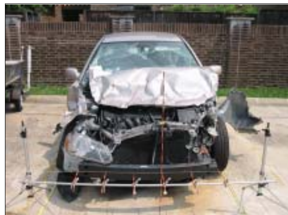
Figure 3: Case vehicle's frontal damage with contour gauge set at bumper level; Note: case vehicle underrode left side of Ford pickup (case photo #18)
