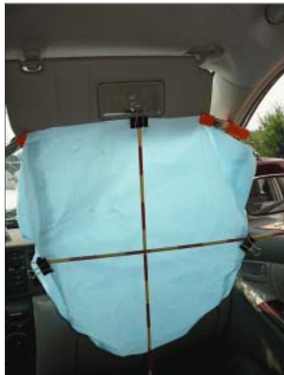
Figure 11: Case vehicle's deployed front right passenger air bag showing no occupant contact evidence (case photo #59)
