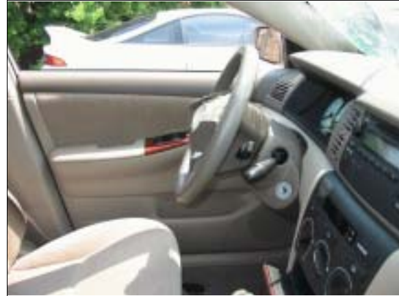
Figure 9: Case vehicle's driver seating area viewed from right showing no deformation to steering wheel or other obvious occupant contact evidence (case photo #51)
