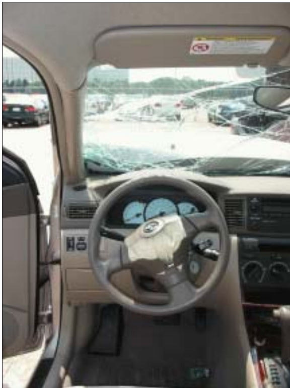
Figure 6: Case vehicle's driver seating and greenhouse areas showing steering wheel-mounted deployed air bag module and no obvious contact evidence to left "A"-pillar, sun visor/windshield header, and/or roof (case photo #44)
