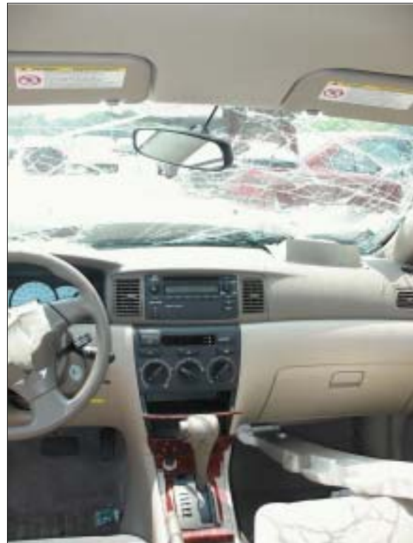
Figure 7: Case vehicle's front instrument panel, center console, sun visors, roof, and windshield's header and glazing; Note: only obvious contact occurred to driver's knee bolster (yellow tape), right of steering column (case photo #45)
