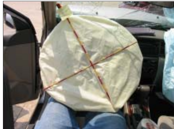
Figure 10: Case vehicle's deployed driver air bag showing no apparent evidence of occupant contact (case photo #52)
