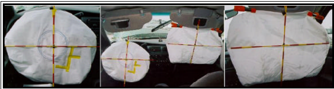
Figure 5. 2000 Ford Taurus SE deployed redesigned frontal air bags.
