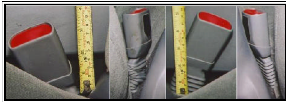
Figure 6. 2000 Ford Taurus SE deployed driver and non-deployed front right buckle pretensioners.
