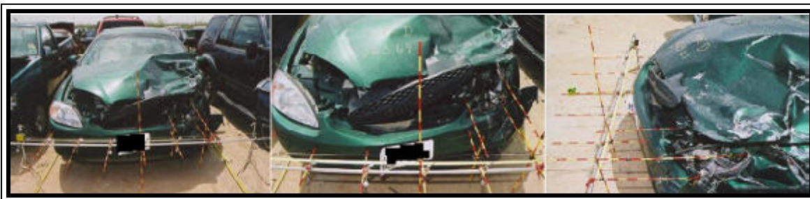
Figure 3. Front left damage to the 2000 Ford Taurus SE.
