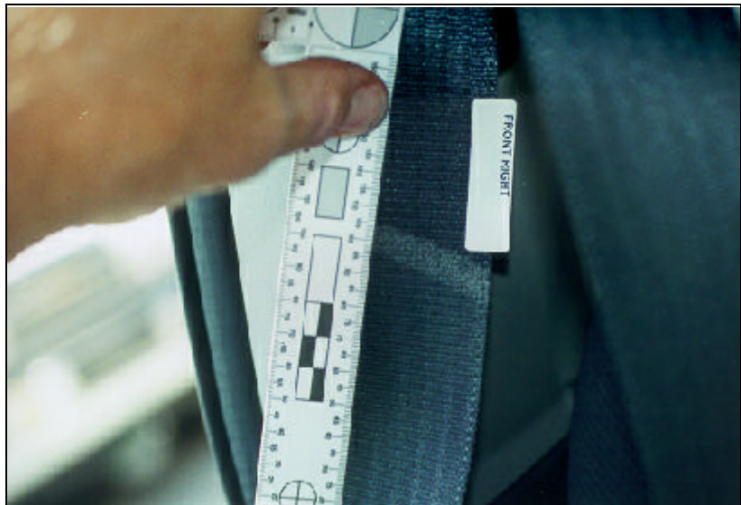
Figure 11. Loading marks, front right seat belt
