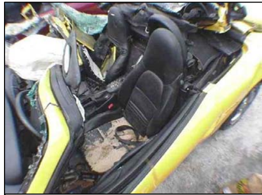
Figure 4 - Driver's seating position, stretched webbing of shoulder belt, deformed front right seat.
