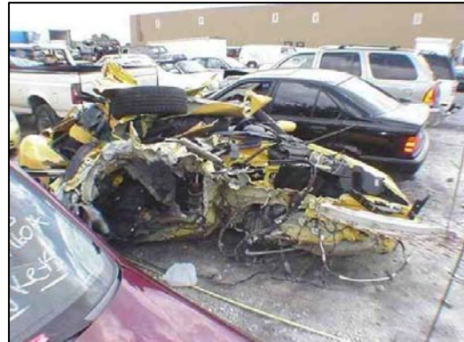
Figure 3 – Right lateral view of the damage profile.
