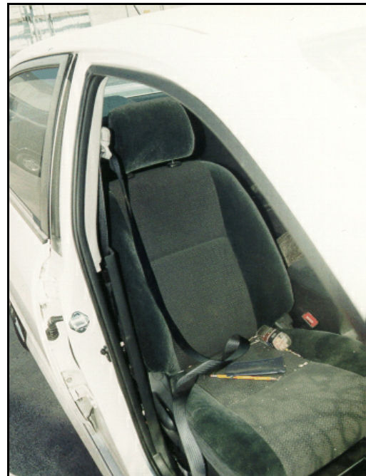
Figure 13. FR occupant's actuated pretensioner and retractor cover displaced
