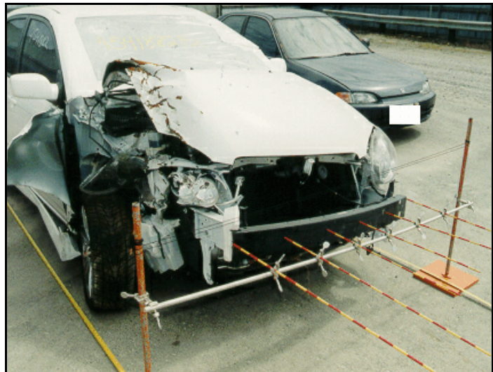
Figure 7. Front exterior damage to case vehicle
