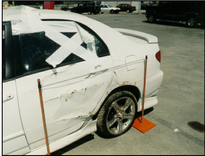
Figure 8. Left rear damage to case vehicle
