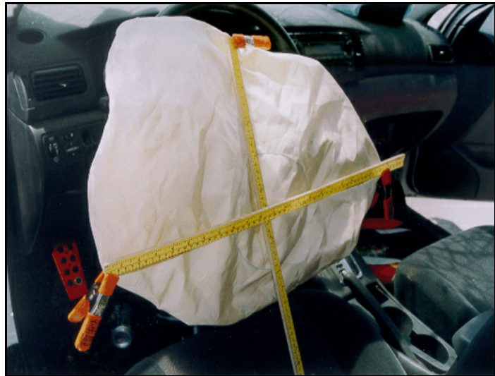
Figure 11. Driver's deployed air bag
