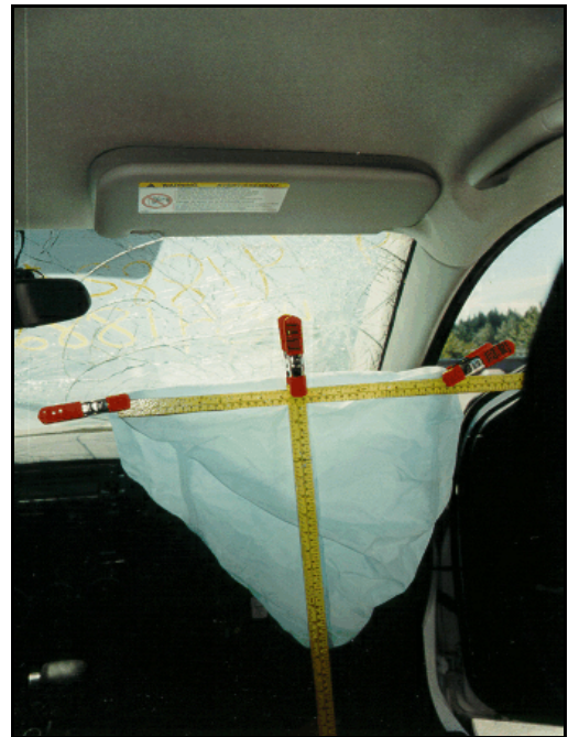
Figure 12. FR occupant's deployed air bag
