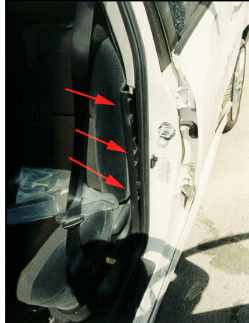
Figure 9. Driver's seat belt actuated pretensioner and retractor displaced
