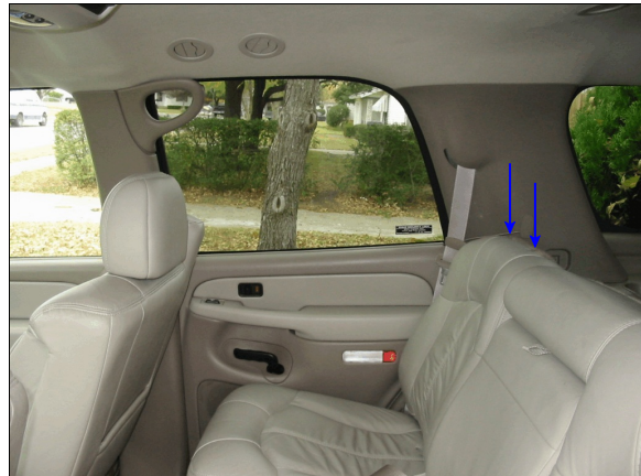
Figure 6: Case vehicle's second seating area showing missing adjustable head restraint (see arrows) for right-most seating position and non-integral safety belt system (case photo #55)
