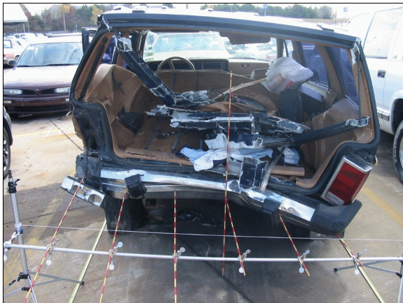
Figure 4: Jeep's back damage with contour gauge present at bumper level; Note: crush to left "D"-pillar and obliterated liftgate and backlite (case photo #72)
