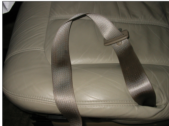
Figure 7: Lap portion of case vehicle's driver integral safety belt anchored within seat cushion (case photo #39)
