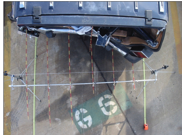
Figure 19: Overhead view of Jeep’s back damage with contour gauge present at bumper level; Note: crush more extensive to back left corner (case photo #71)
