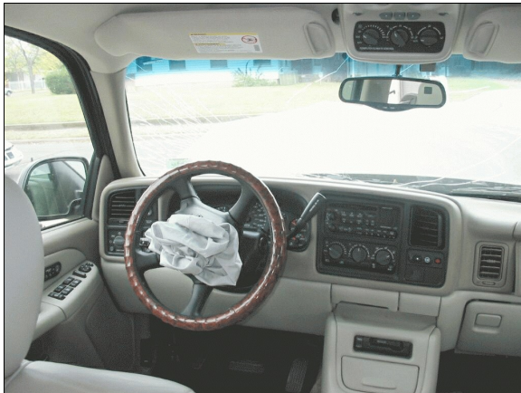
Figure 13: Case vehicle's driver seating area showing no apparent occupant contact evidence on steering wheel, instrument panel, or greenhouse areas (case photo #30)
