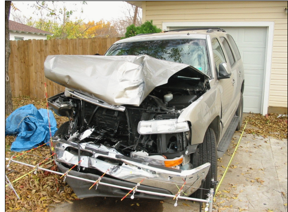
Figure 3: Case vehicle's frontal damage viewed from left of front with contour gauge present at bumper level; Note: rightward offset nature of impact, resulting in rightward shift of hood and more crush to front right corner (case photo #15)
