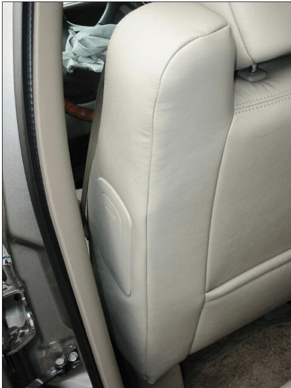
Figure 9: Case vehicle's non-deployed left front seat back-mounted side impact air bag (case photo #37)
