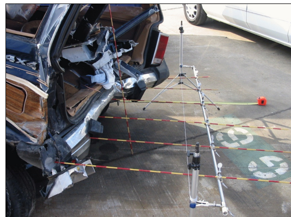
Figure 20: Jeep’s back damage viewed along reference line from left with contour gauge present at bumper level showing crush profile; Note: crush more extensive to back left corner (case photo #69)
