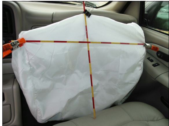
Figure 16: Front surface of case vehicle's front right passenger air bag showing no apparent evidence of occupant contact (case photo #48)
