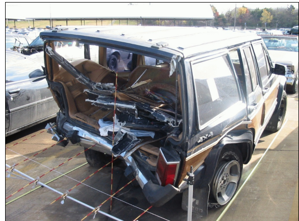
Figure 5: Jeep's back damage viewed from right of back with contour gauge at bumper level showing leftward offset nature of impact, greater crush to back left corner, and damaged left "D"-pillar (case photo #73)
