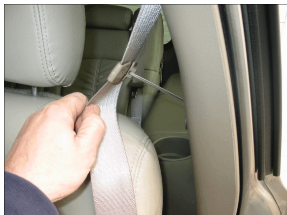
Figure 8: Tether attached to torso portion of Case vehicle's second seat left safety belt; Note: integral safety belt for back left seating position in background (case photo #56)
