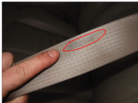
Figure 18: Slight scuff/burn on webbing of shoulder belt portion of case vehicle's driver safety belt (case photo #38)
