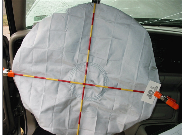
Figure 15: Front surface of case vehicle's deployed driver air bag showing no apparent evidence of occupant contact; Note: steering wheel rim is rotated approximately 90 degrees clockwise (case photo #41)
