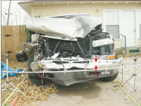
Figure 2: Case vehicle's frontal damage with contour gauge present at bumper level; Note: rightward shift to hood, slight upward rotation of front bumper, and yellow tape (arrows) marks width of direct damage on bumper (case photo #06)
