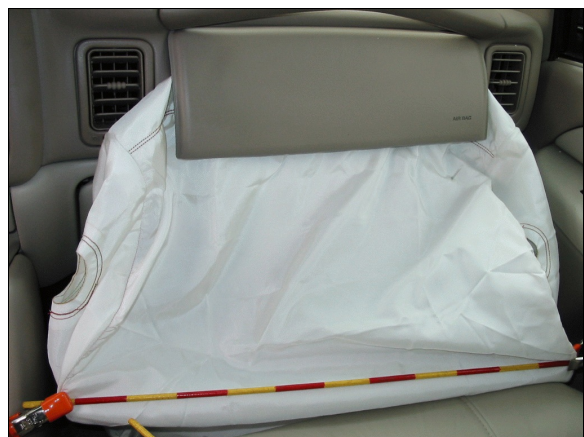
Figure 17: Top surface of case vehicle's deployed front right passenger air bag showing no apparent evidence of occupant contact to top surface or air bag module's cover flap (case photo #49)
