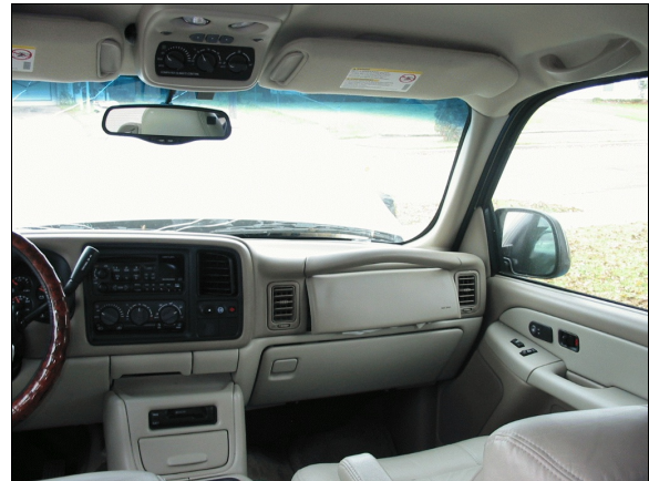
Figure 14: Case vehicle's front right seating area showing no apparent driver contact evidence to center console, instrument panels, or greenhouse areas (case photo #32)
