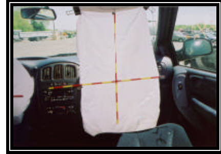
Figure 10. Deployed front right passenger's air bag
