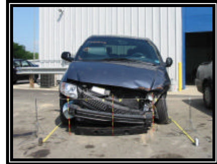
Figure 4. Frontal damage to the Dodge Caravan
