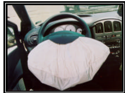
Figure 8. Driver’s air bag cover flap
