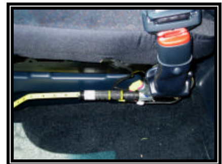
Figure 7. Front right buckle pretensioner
