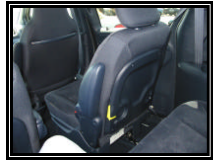
Figure 6. Scuff on the rear aspect of the second row right seat back
