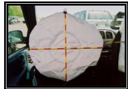
Figure 9. Deployed driver’s air bag
