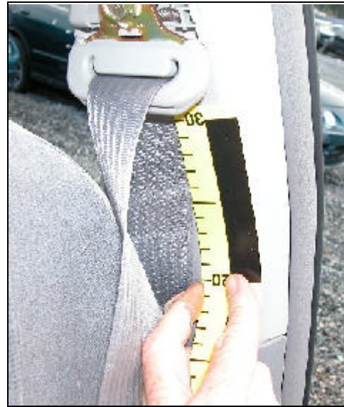
Figure 9. Scuffing to driver's seatbelt
