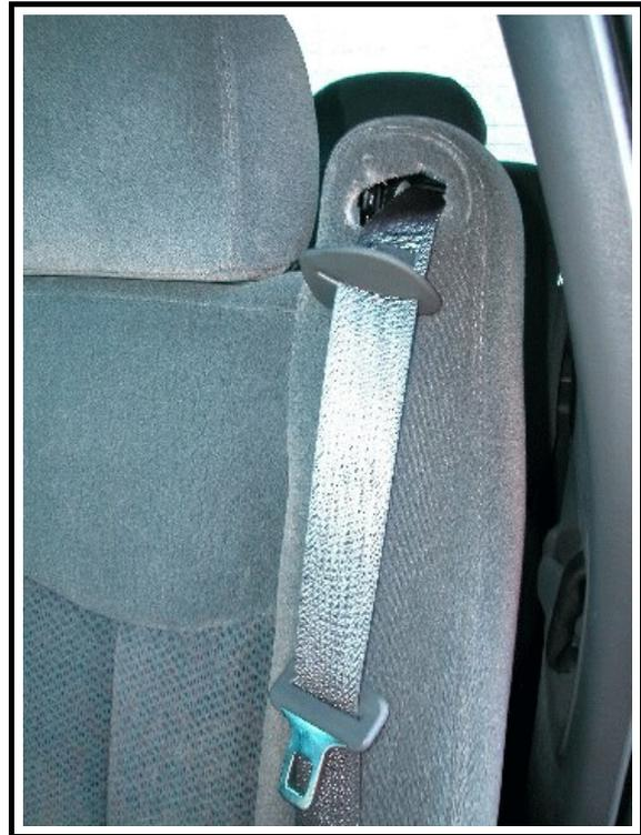
Figure 4. Driver's displaced plastic cover
