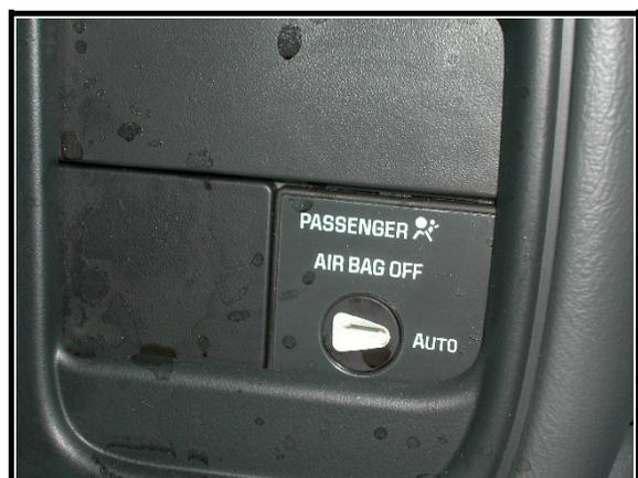
Figure 7. Front right passenger air bag cut off switch
