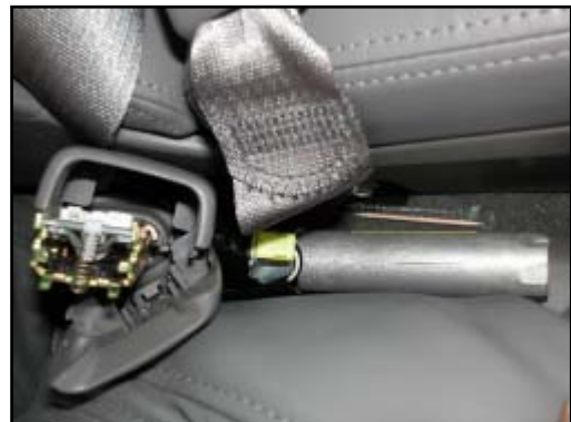
Figure 11. View of front right passenger's buckle pretensioner and fractured buckle housing
