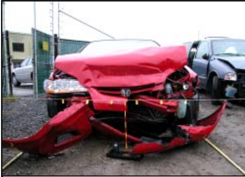
Figure 4. Frontal damage to the 2001 Honda Accord
