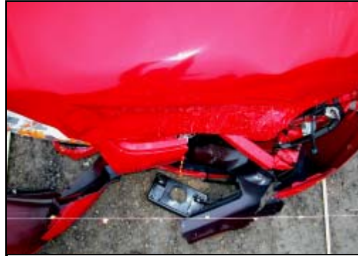
Figure 5. View showing crushed bumper beam
