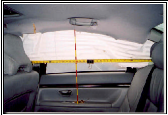
Figure 21: Left interior view of the deployed inflatable curtain at the rear right position.
