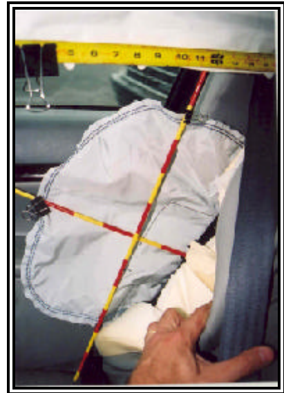
Figure 19: View of the deployed right side impact air bag.
