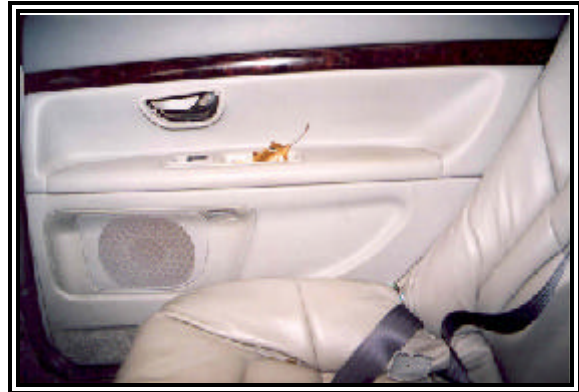
Figure 16: View of the rear right intrusion and seat compression.
