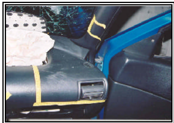
Figure 8: Air bag transfers to the right aspect of the IP.
