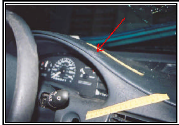
Figure 10: Contact evidence to the IP brow.
