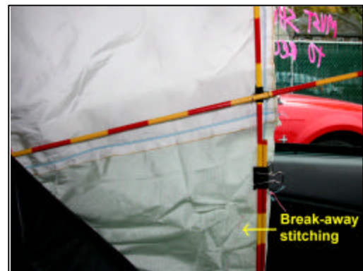
Figure 10. View of center seam and vertical break-away stitching
