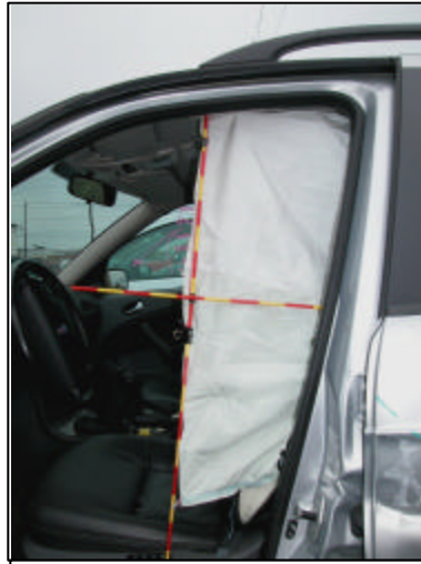
Figure 9. View of outboard aspect of the driver's side impact air bag
