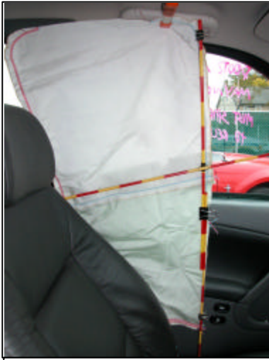
Figure 8. View of inboard aspect of the driver's side impact air bag
