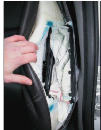
Figure 11. View of plastic air bag module housing located behind the seat back tear seam
