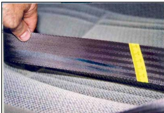
Figure 10 - Loading evidence on driver's shoulder belt webbing.
