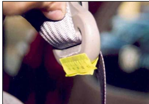
Figure 11 - Loading evidence on left front D-ring.
