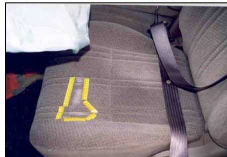
Figure 7 - Frictional abrasion to driver's seat cushion.
