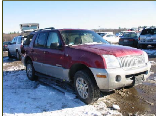
Figure 7. Rollover damage to the right to the right front fender, right running board, right rear quarter window, and D-pillar.
