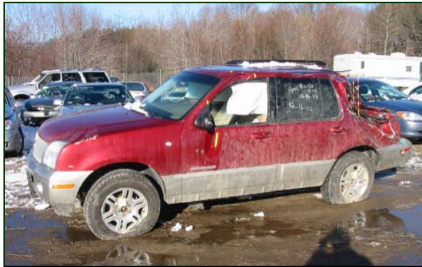
Figure 5. Left side rollover damage to the Mounatineer.
