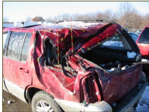
Figure 6. Rock impact damage to the roof, backlight header, D-pillar area of the vehicle.
