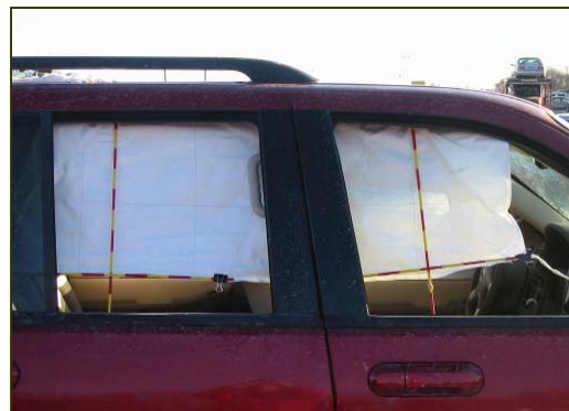
Figure 10. Overall view of the deployed right side rollover canopy air bag.
