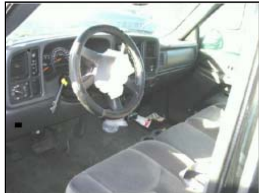
Figure 6. Interior view of front row. Note contact damage to turn signal lever.
