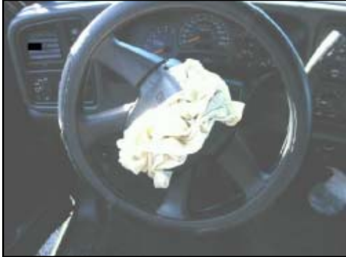
Figure 8. Deployed front left air bag.
