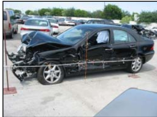
Figure 5. Left side damage from impact with the BMW.
