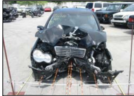
Figure 6. Pole impact damage to the front center area of the Mercedes-Benz.
