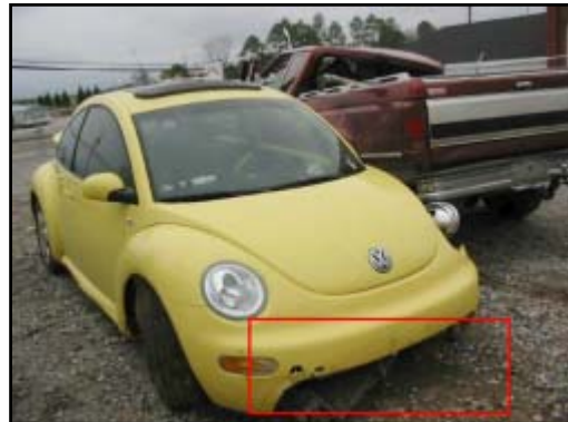
Figure 8. Frontal damage from the second culvert impact.
