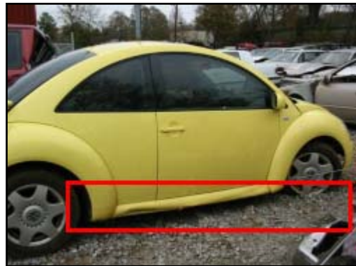
Figure 7. Residual damage from the first culvert impact.
