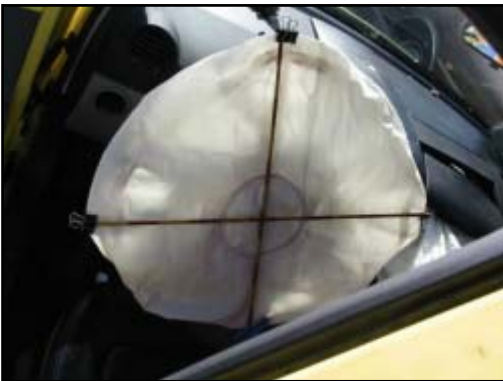
Figure 13. Deployed driver's frontal air bag. Note the steering wheel is rotated 180 degrees therefore the top of the air bag is at the bottom of the picture.
