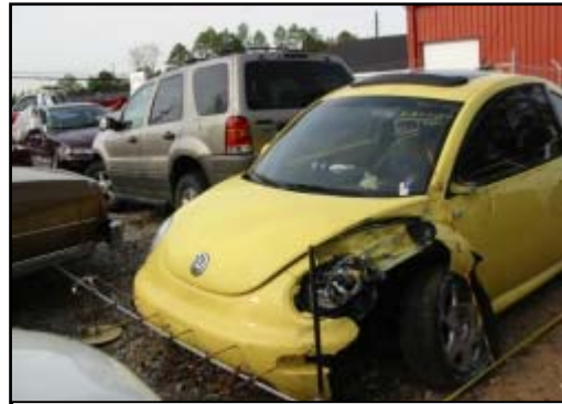
Figure 6. Damage from the impact with the Mercury.
