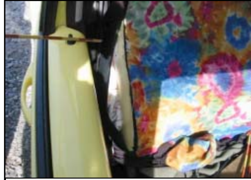
Figure 12. Side impact air bag cover flap. Note the aftermarket seat cover seam and the seam of the seat appear to overlap.
