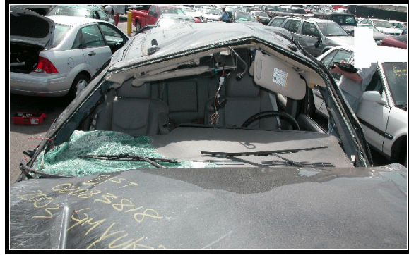
Figure 9. Front view of case vehicle showing windshield and roof rail intrusions
