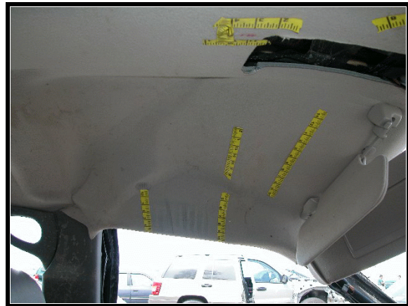
Figure 10. Driver contacts to roof, roof rail, and header
