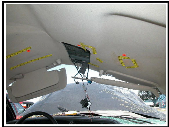
Figure 16. Contacts to the roof and header area
