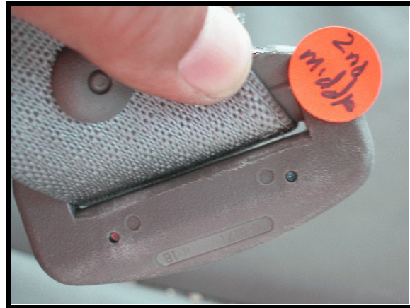
Figure 14. Load marks to middle rear seat belt latch
