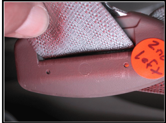
Figure 13. Load marks to left rear seat belt latch
