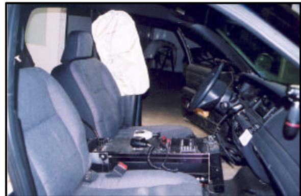
**Figure 7: Right interior view depicting the deployed side impact air bag.**
