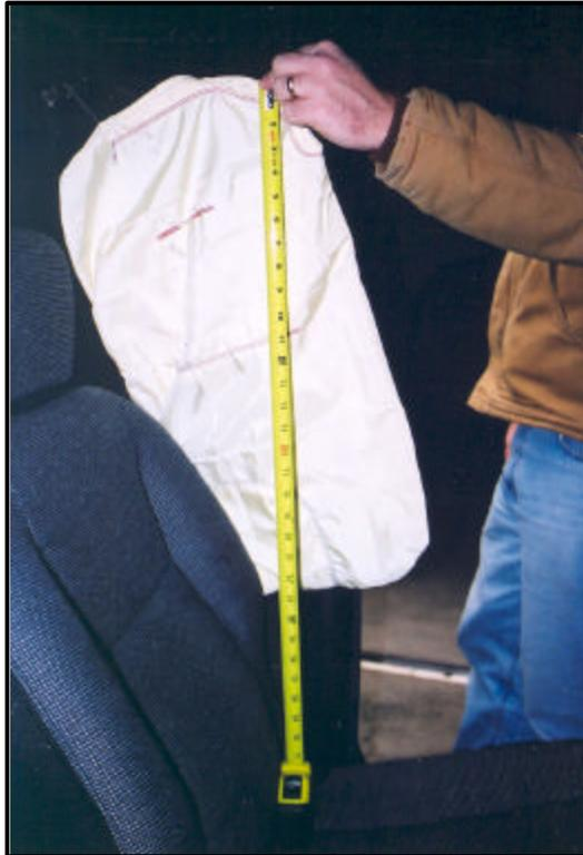
**Figure 8: Deployed side impact air bag.**
