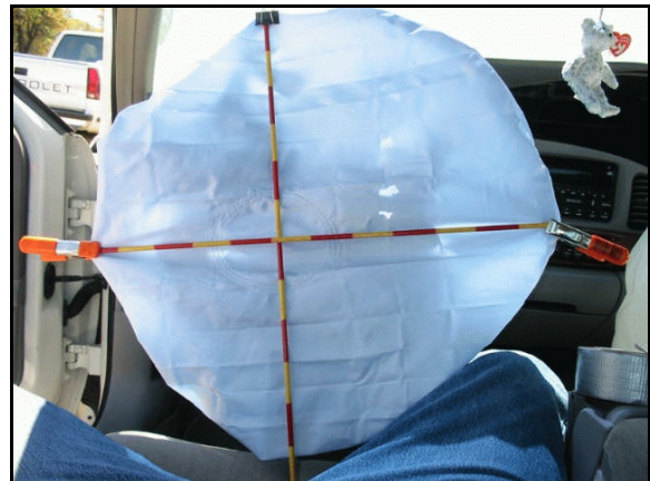
Figure 4: Front of driver's air bag (case photo #40)
