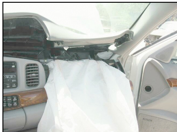
Figure 5: Deployed front right passenger air bag, showing displaced top of "active instrument panel" (case photo #49)
