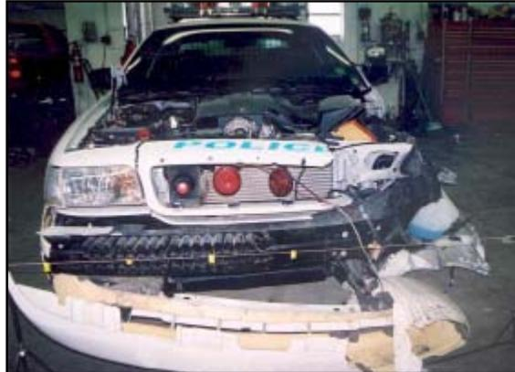
**Figure 3. Resultant frontal damage to the Ford.**
