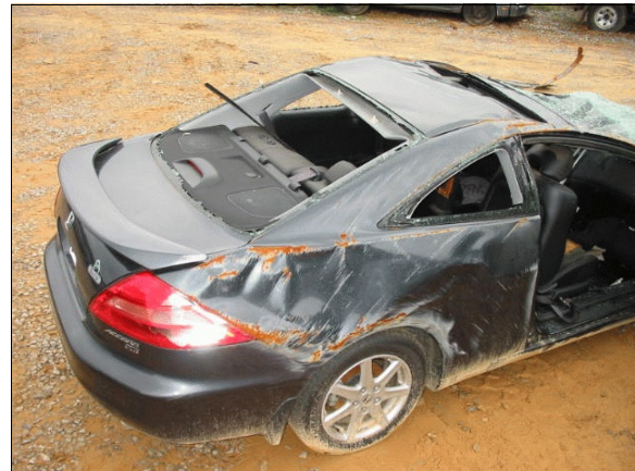
Figure 5: Rollover damage to case vehicle's right quarter panel, front door, roof side rail, and "A"-pillar; Note: backlite and right side glazing disintegrated (case photo #21)
