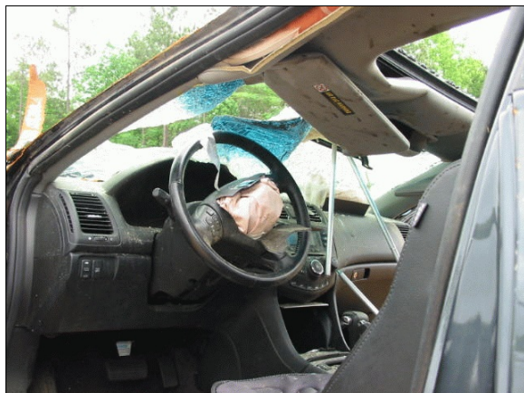
Figure 11: Case vehicle's driver seating area viewed from left at seat level; Note: blood splatter to driver's sun visor and roof and exposed, non-deployed, left side-inflatable curtain air bag (case photo #27)
