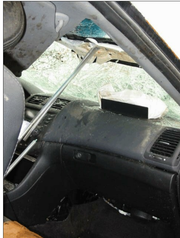
Figure 16: Case vehicle's top-mounted front right passenger air bag showing lower cover flap and no obvious contact evidence to front right knee bolster or glove box (case photo #45)
