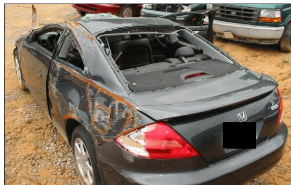
Figure 4: Elevated view from left of back showing rollover damage to case vehicle's left quarter panel and roof side rail (case photo #20)
