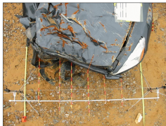
Figure 8: Overhead view of case vehicle’s frontal crush from impact with back of Plymouth; Note: contour gauge at bumper level and hood damage from subsequent rollover impact (case photo #18)
