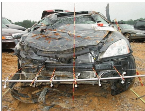
Figure 2: Case vehicle's frontal damage viewed at bumper level with contour gauge present; Note: damage primarily to right half (case photo #06)
