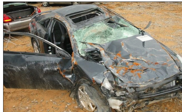
Figure 6: Elevated view from right of front of showing extensive rollover damage to case vehicle's top and right side (case photo #22)
