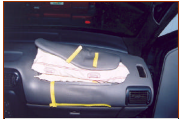
Figure 8: View of the deformed cover flap.
