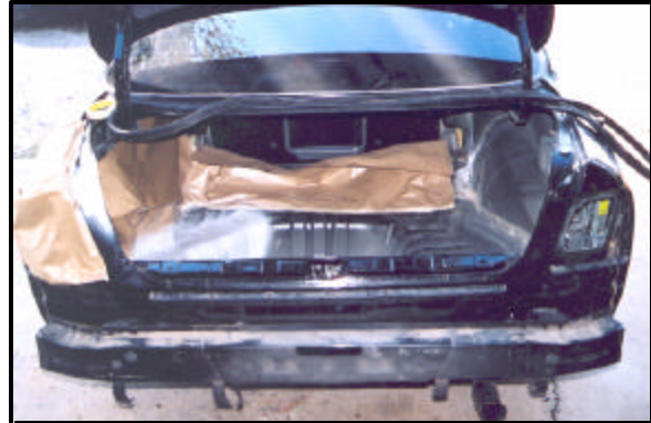
Figure 6: View of the repaired trunk well.
