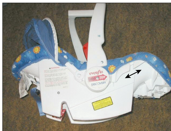
Figure 19: Left (inboard) side of Evenflo Discovery infant safety seat used in rear-facing position by case vehicle’s back right passenger; Note: arrow marks safety belt path (case photo #51)
