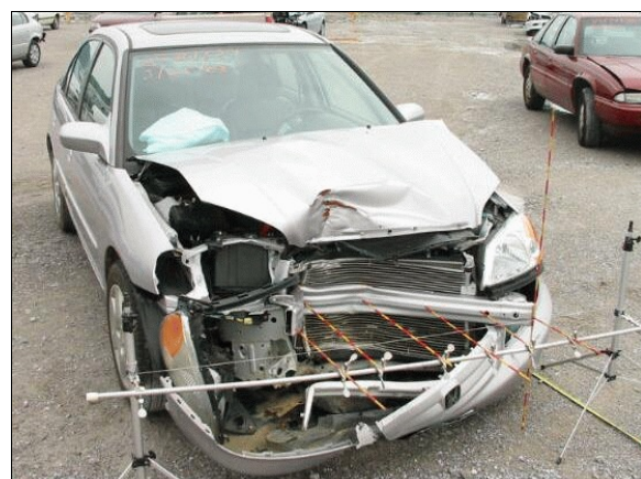
Figure 8: Elevated view of case vehicle's frontal damage with contour gauge set at bumper level, viewed from right of front (case photo #21a)
