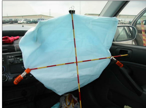
Figure 16: Case vehicle's deployed front right passenger air bag showing no occupant contact evidence (case photo #41)
