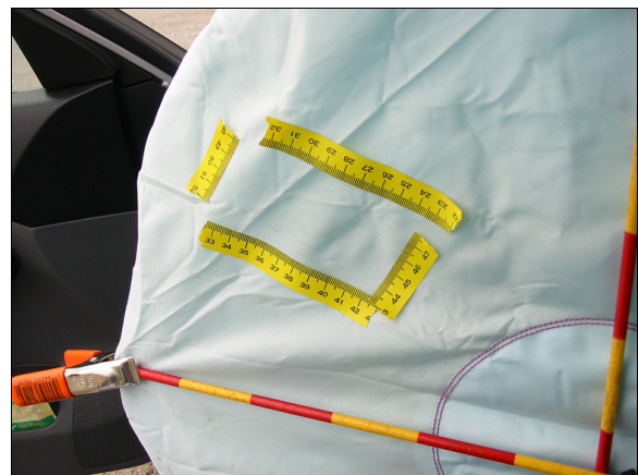
Figure 15: Close-up of occupant contact evidence on case vehicle's driver air bag (case photo #29)
