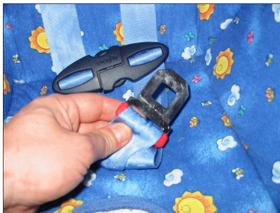
Figure 23: Loading evidence on latch plate of Evenflo Discovery infant child safety seat used by case vehicle's back right passenger (case photo #55)
