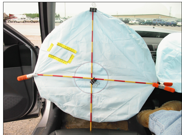
Figure 14: Case vehicle's deployed driver air; Note: yellow tape highlights area of occupant contact (case photo #28a)
