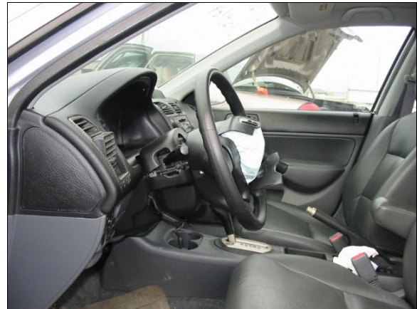
Figure 13: Case vehicle's driver seating area, viewed from driver's door, showing loading to steering column (case photo #25)
