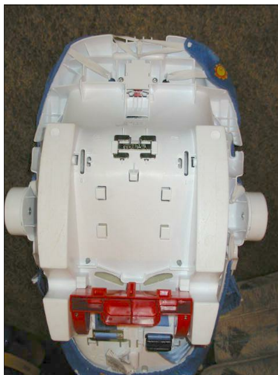
Figure 18: Back surface of Evenflo Discovery infant child seat used by case vehicle’s back right passenger; Note: no visible evidence of damage (case photo #52)
