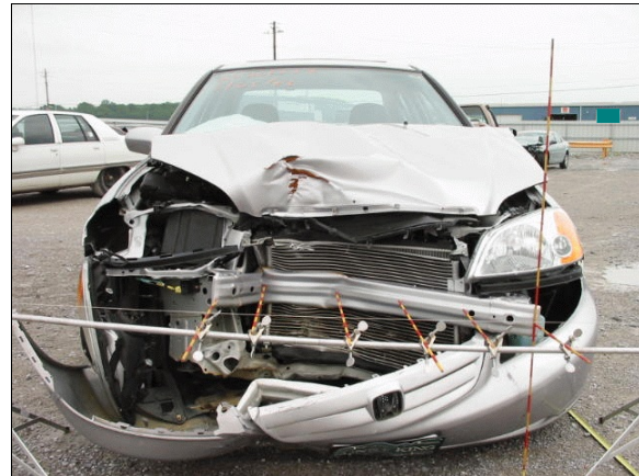
Figure 6: Case vehicle's frontal damage with contour gauge set at bumper level (case photo #10)
