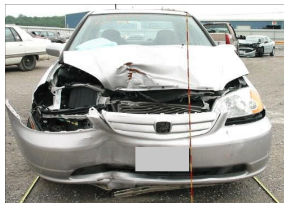
Figure 5: Case vehicle’s frontal damage with bumper fascia placed in approximate post-crash position (case photo #09)
