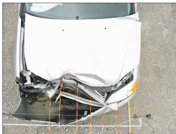
Figure 9: Overhead view of case vehicle’s frontal damage pocket from tree impact and crush profile measured at bumper level (case photo #10a)
