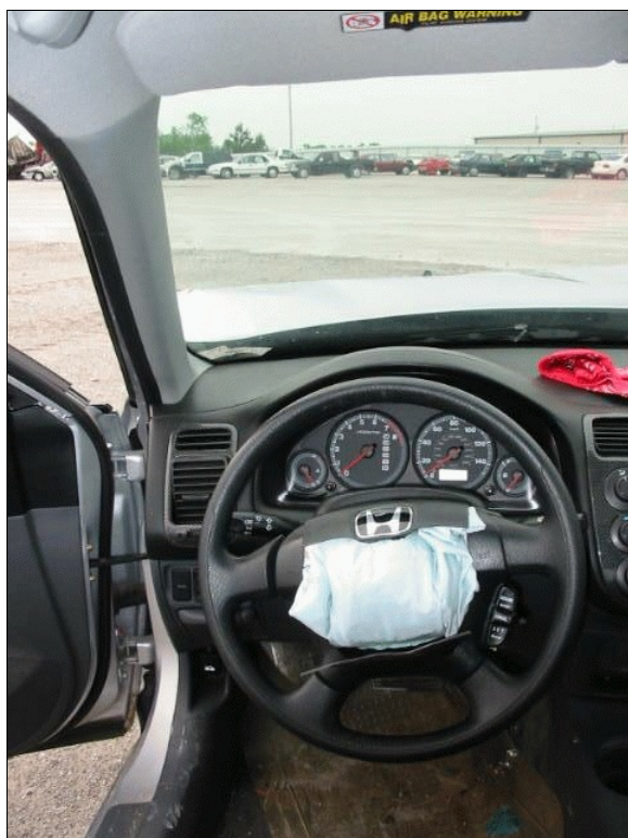
Figure 10: Vertical view of case vehicle's driver seating area showing deployed driver air bag and no obvious contact evidence to greenhouse area (case photo #27)
