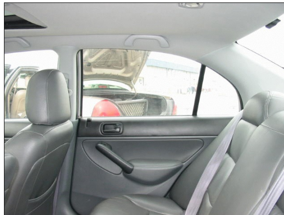
Figure 21: Case vehicle's back right seating area, view from left rear door, showing no obvious contact evidence from infant child seat (case photo #45)
