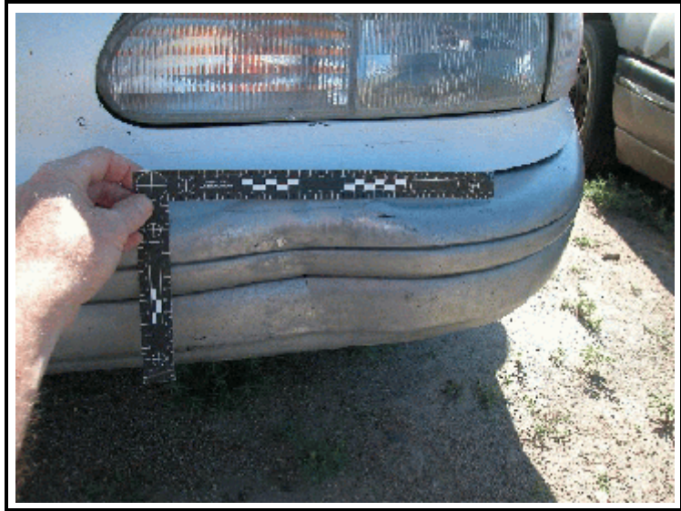
Figure 7. Close up of minor damage to bumper
