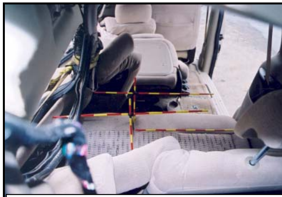
Figure 14: Forward view of the third row intrusion.
