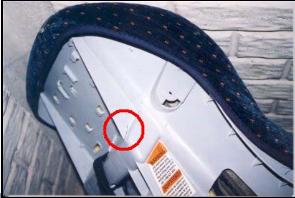
Figure 18: View of damage to the back of the CSS shell.
