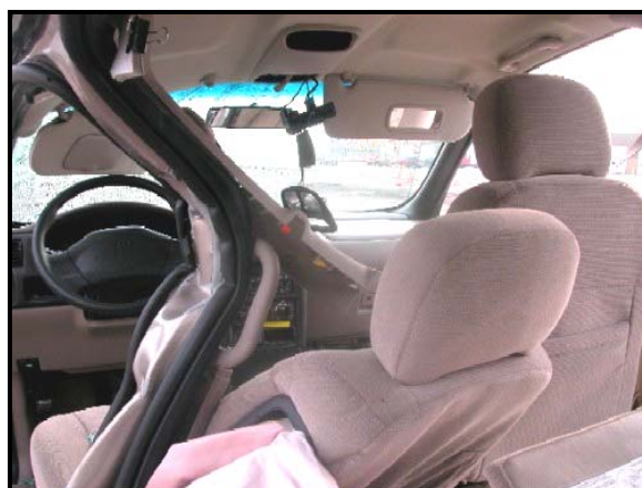
Figure 10: Driver seat deformation and left B-pillar intrusion.
