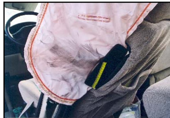
Figure 16: Close-up view of the impeded SAB.
