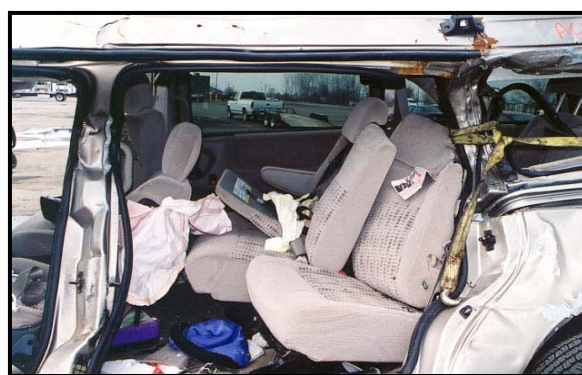
Figure 11 View of the second row seat deformation and intrusion.
