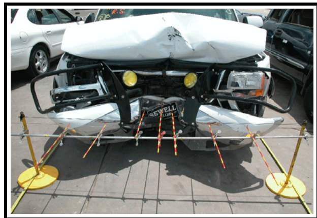
Figure 5. View of case vehicle showing frontal deformation (maximum crush depth 48.2 cm)
