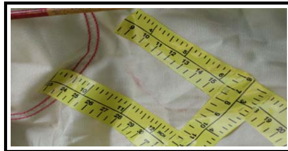
Figure 8. Close-up view of the driver's air bag showing lipstick/cosmetic transfer
