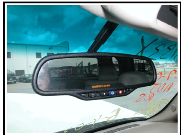
Figure 6. Close-up view showing passenger air bag sensing system and OnStar
