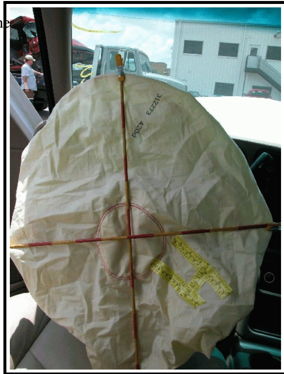
Figure 7. View showing deployed front, left (drivers) air bag
