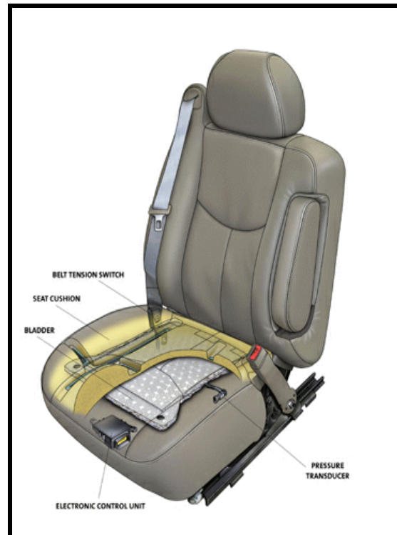
Figure 9. Front right Passenger Sensing System
