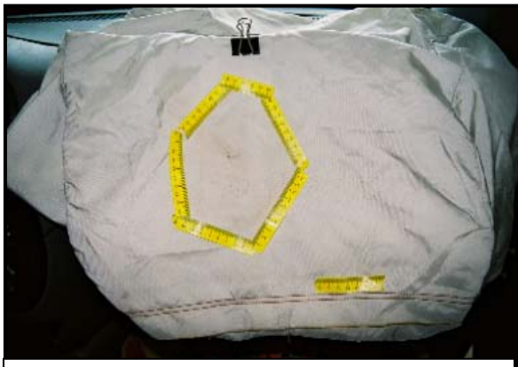
Figure 16: Contact to the bottom surface of the PAB.
