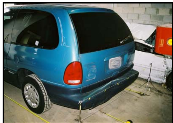
Figure 4: Rear bumper deformation.
