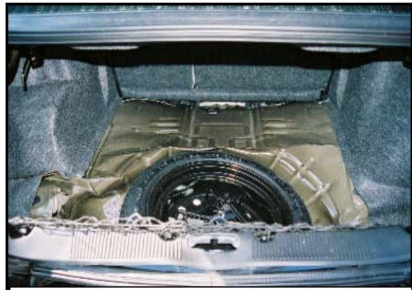
Figure 6: View of the trunk collapse.
