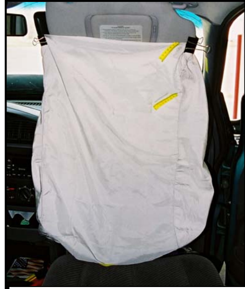
Figure 135: View of the face of the PAB.
