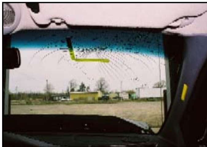
Figure 11: View of the windshield fracture and abraded A-pillar trim.
