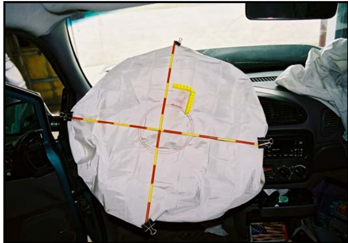
Figure 12: Driver air bag. Note, the steering wheel is rotated 180 degrees.
