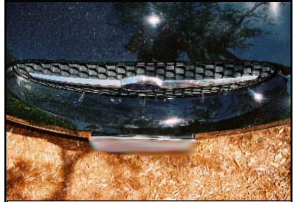
Figure 8: Abrasions to the center section of the fascia.
