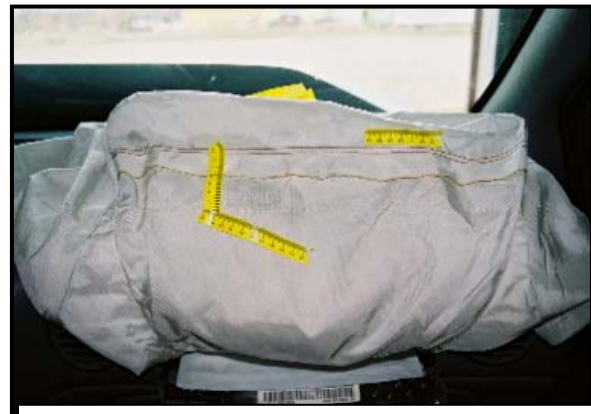
Figure 17: Contact to the bottom surface of the PAB.
