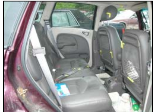
Figure 13. View of damage to the front seat backs
