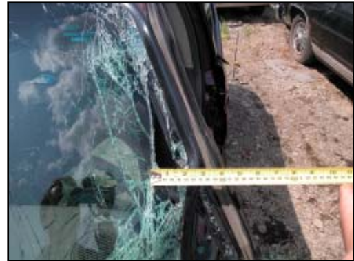
Figure 11. View of torn windshield laminate and left A-pillar displacement
