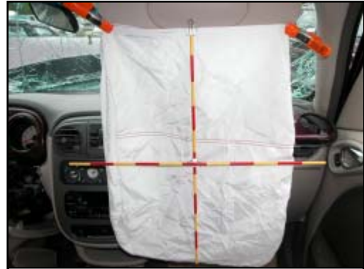
Figure 22. Redesigned front right passenger's air bag
