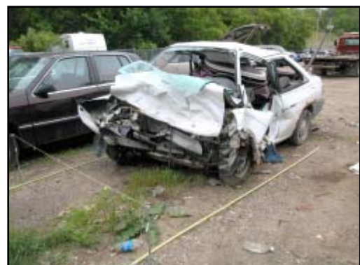
Figure 8. View of frontal damage to the Ford Escort
