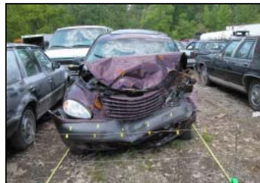
Figure 5. View of frontal damage to the PT Cruiser
