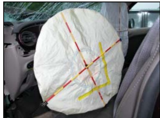
Figure 21. Deployed redesigned driver's air bag showing makeup transfer
