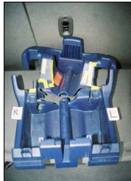
Figure 20. View of fractured CSS base
