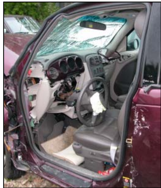
Figure 12. View of collapsed steering column, rim deflection, and interior damage to the driver's seating position
