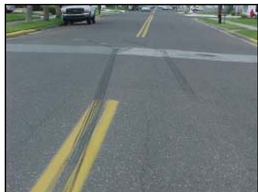
Figure 6. Police photograph of pre-impact tire marks from the CVPI showing deflection points and final rest
