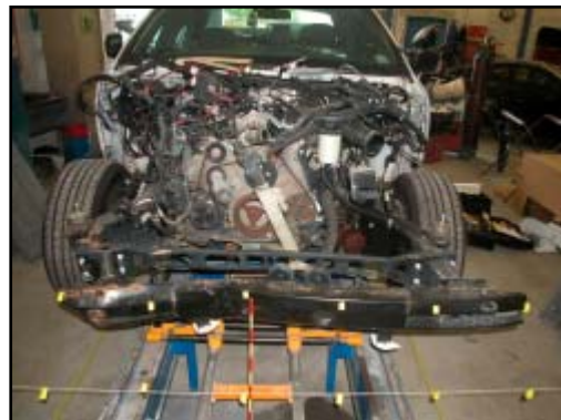
Figure 8. Frontal view showing damaged/shifted bumper beam
