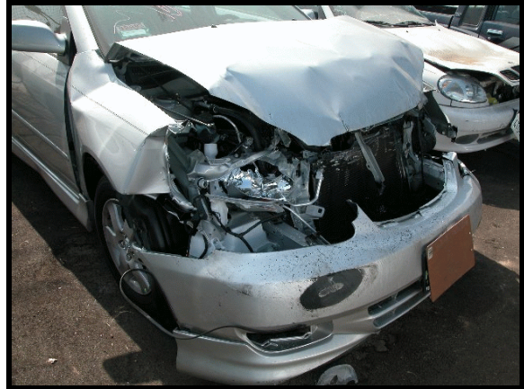
Figure 1. Front, right view of case vehicle showing significant underide deformation
