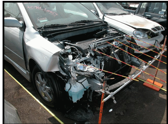
Figure 4. View of case vehicle with hood and fascia removed exposing the extent of upper bumper deformation
