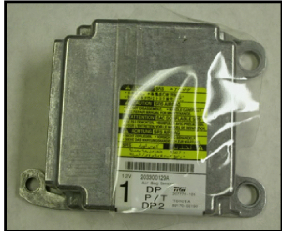
Figure 7. Air bag sensor module (EDR)
