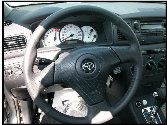
Figure 6. View showing non-deployed steering wheel hub mounted air bag
