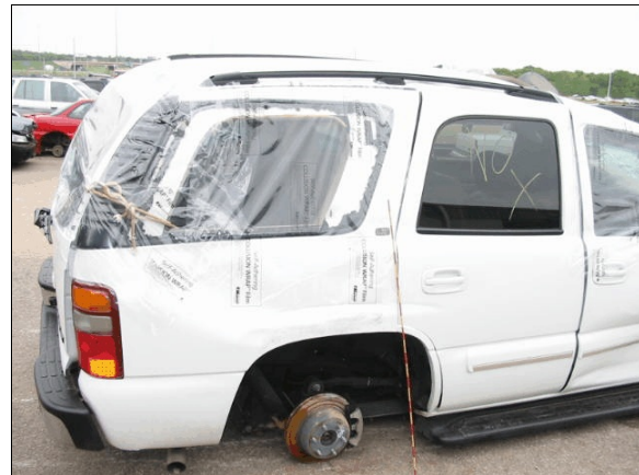
Figure 11: Rollover damage to case vehicle's right quarter panel and doors, including disintegrated right front door and 2 nd right rear window glazings and remote buckling to doors and quarter panel (case photo #31)
