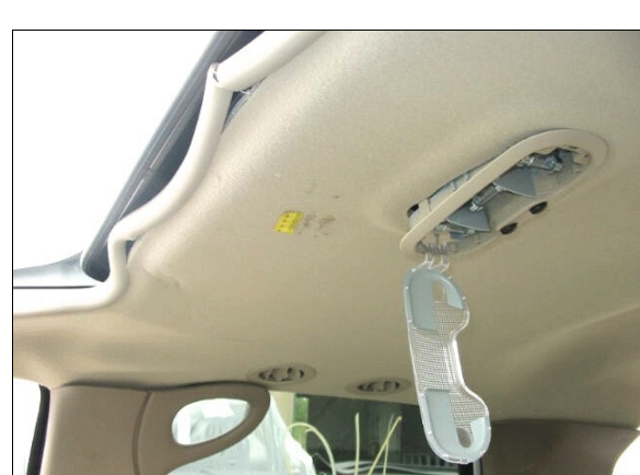
Figure 18: Contact evidence on case vehicle’s roof situated between moon roof and damaged dome light (case photo #52)
