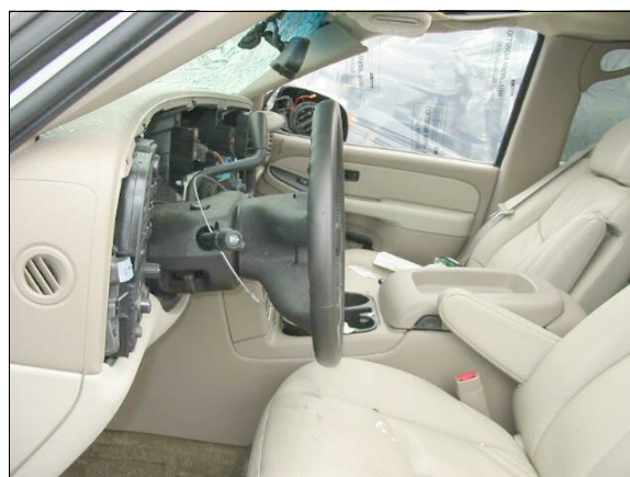
Figure 14: Case vehicle’s front seating area showing no deformation to steering wheel rim, driver’s armrest bent toward center console, and angulation of front seat backs (case photo #42)
