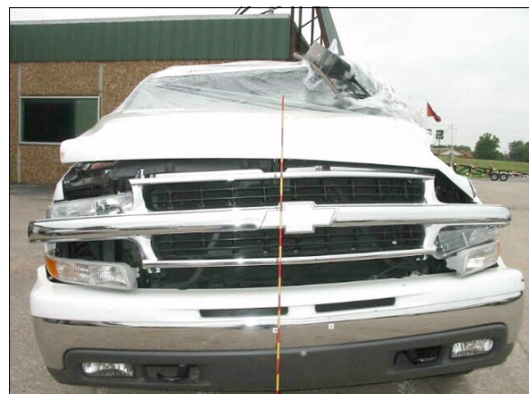
Figure 12: Case vehicle viewed from front bumper level showing greatest roof crush occurred along right roof and right "A"-pillar and induced damage to front and hood (case photo #22)
