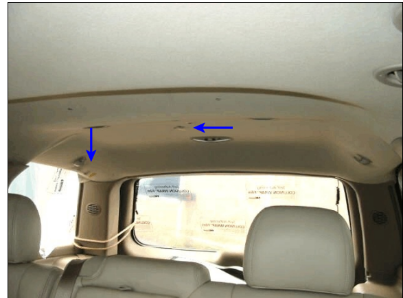
Figure 20: Oblique view of case vehicle's interior indicating driver's suspected front left to back right path of movement during rollover; Note: arrows show possible occupant contact locations (case photo #54)
