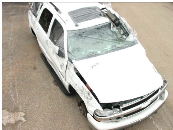
Figure 7: Elevated view of rollover damage to case vehicle's right side (case photo #37)
