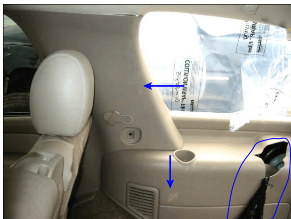
Figure 23: Right interior surface of case vehicle's back right seating area showing disintegrated 2 nd right window glazing and contact evidence on interior surface, probably related to an interior loose object (case photo #57)
