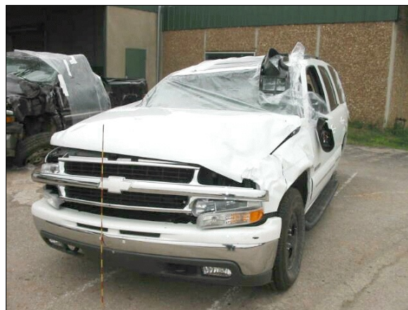
Figure 8: Rollover crush to case vehicle's left fender and front left hood viewed from left of front; Note: greater crush to right roof and right "A"-pillar and damaged left outside rearview mirror (case photo #23)
