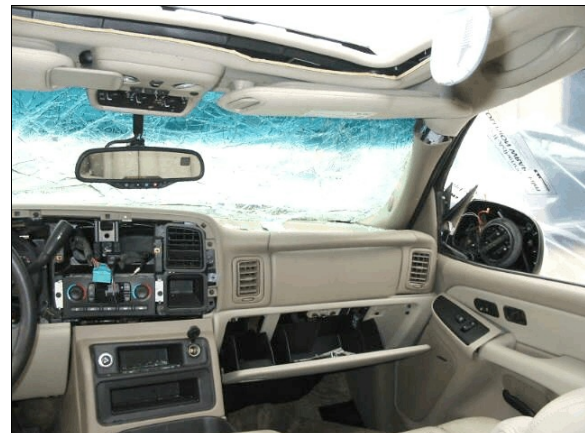
Figure 16: Case vehicle’s front right seating area showing non-deployed front right passenger air bag, cracked windshield, altered center instrument panel, and no obvious occupant contact evidence (case photo #45)
