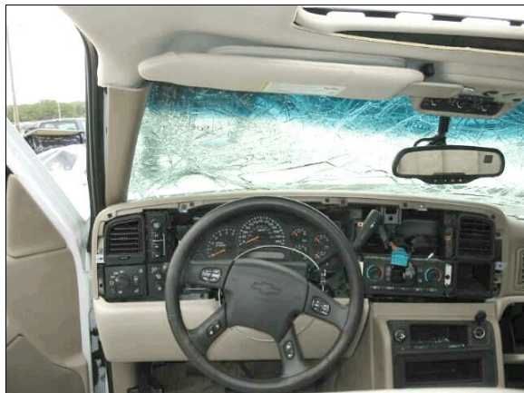
Figure 15: Case vehicle’s driver seating area showing non-deployed driver air bag, cracked windshield’s glazing, and removed center instrument panel molding; Note: no obvious evidence of occupant contact (case photo #43)
