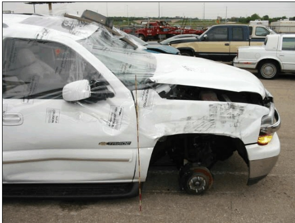
Figure 10: Rollover damage to case vehicle's right fender, lower right front door, right outside rearview mirror, right "A"-pillar, and right hood; Note: right front wheel missing (case photo #36)
