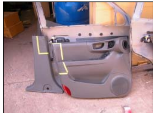
Figure 7. Damaged interior left front door panel and left B-pillar trim
