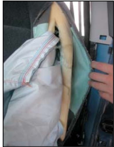
Figure 11. View of the outboard seat back and tear seam showing foam and interior liners
