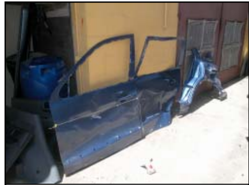
Figure 6. View of deformation to both removed left side doors and left quarter panel
