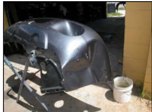
Figure 4. Left front view of damaged bumper fascia
