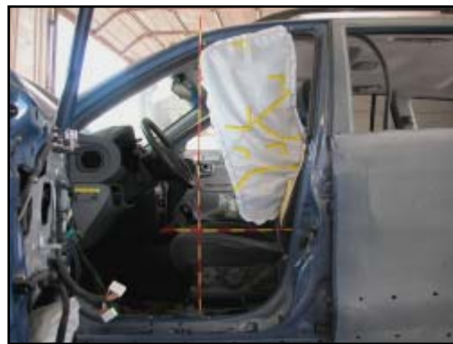
Figure 13. Outboard view of deployed driver's side impact air bag
