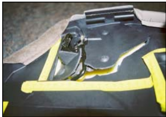
Figure 19. Close-up of right side locking tab and related fracture
