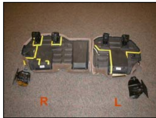
Figure 17. View of bottom aspect of the damaged rear seat and receiver brackets
