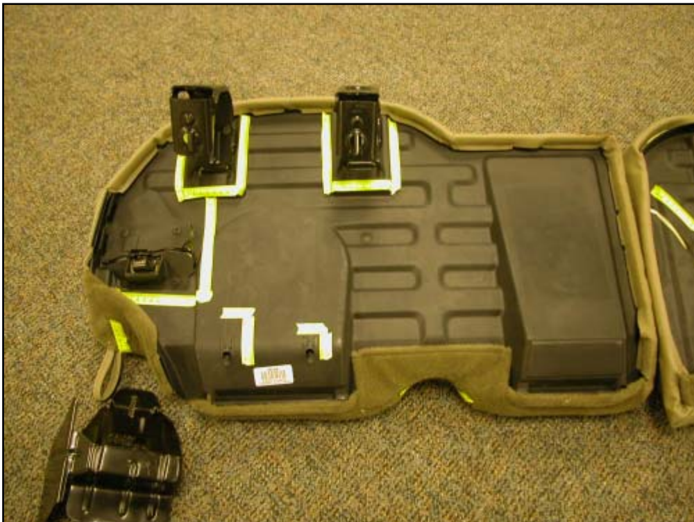
Figure 21. Close-up of damaged right/center seat bottom and receiver bracket
