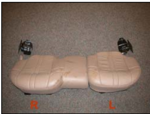
Figure 16. View of top aspect of the damaged rear seat and receiver brackets
