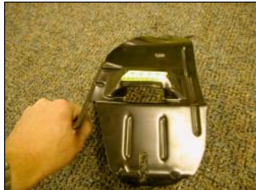
Figure 22. Close up of deformed left receiver bracket
