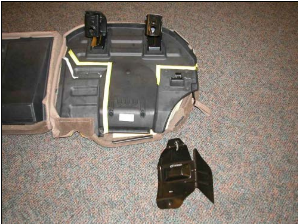
Figure 20. Close-up of damaged left seat bottom and receiver bracket
