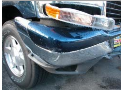
Figure 8. Damage from impact with Ford.
