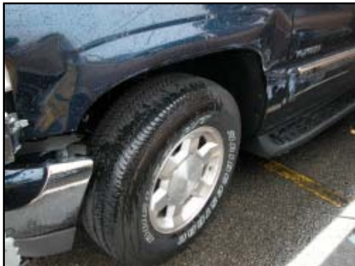
Figure 7. Sideswipe damage from second impact with the Toyota.
