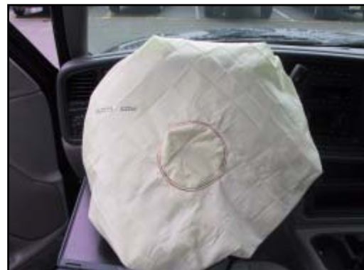
Figure 9. Deployed driver's frontal air bag.
