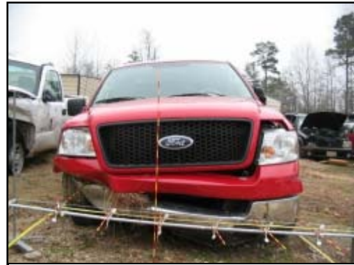
Figure 8. Frontal damage from the ditch impact.
