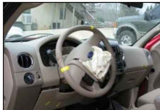
Figure 9. Left knee bolster contacts.
