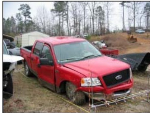
Figure 6. Front right damage from the first W-beam guardrail impact.
