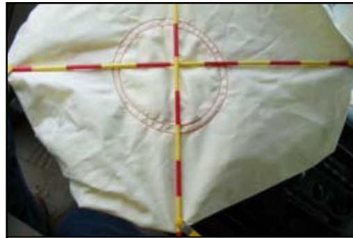
Figure 11. Lower aspect of the deployed driver's air bag.
