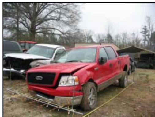
Figure 7. Front left and left side damage from the second W-beam guardrail impact.
