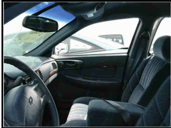
Figure 5. Non deployed front air bags in case vehicle
