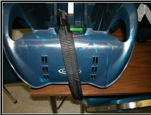
Figure 20. Fractures to front of child seat base.
