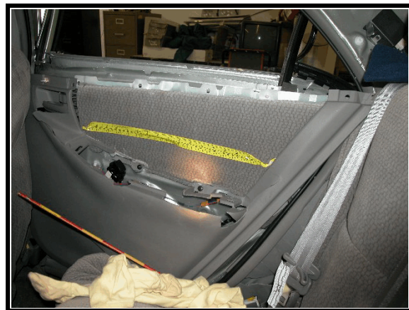
Figure 27. Damage to right rear door side panel due to impact, intrusion, and contact with infant safety seat
