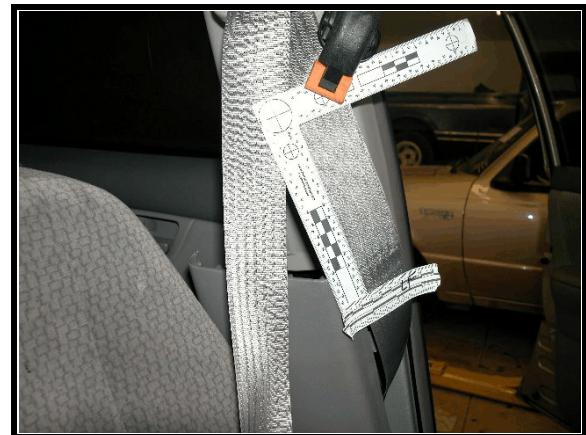
Figure 12. Load marks to driver's seat belt
